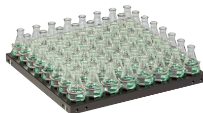
18 x 18", 50 ml Erlenmeyer flask platform Model No. 3524-3
